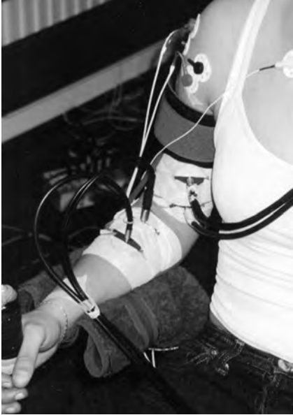
Figure 1.4 In NIRS measurements, two fibre optic cables (optodes) are placed on the skin above the muscle; one for the incoming light and one for the outgoing light. In this way information on the oxygenation of the muscle can be obtained.
