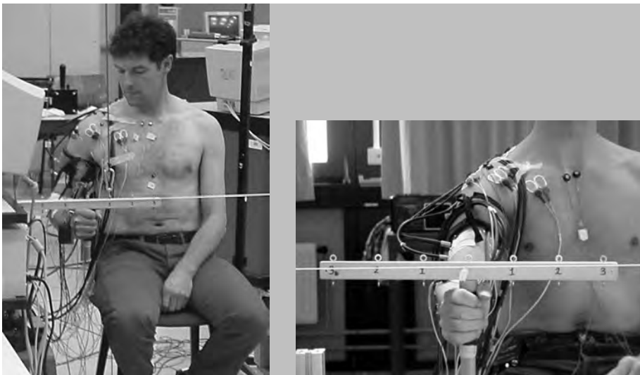
Figure 5.1 Experimental set-up. Subject was sitting on a chair with the elbow flexed and forearm in a horizontal and neutral position. The subject had to hold the tool with his right hand, keeping the bar on top horizontal (a). Visual feedback on the position of the tool was given by a horizontal cord. Flexion moments were enforced by hanging weights right under the stick while extension moments were enforced by loads applied to the middle of the bar using a pulley system. Pro/supination moments were imposed by hanging weights on different distances left or right from the stick (b).
