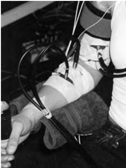
Figure 2.3 NIRS data were measured with fibre optic cables that were attached to the skin above BB and the BR. EMG electrodes were placed on the skin between the cables. A cuff around the upper arm was used to apply an arterial occlusion.
