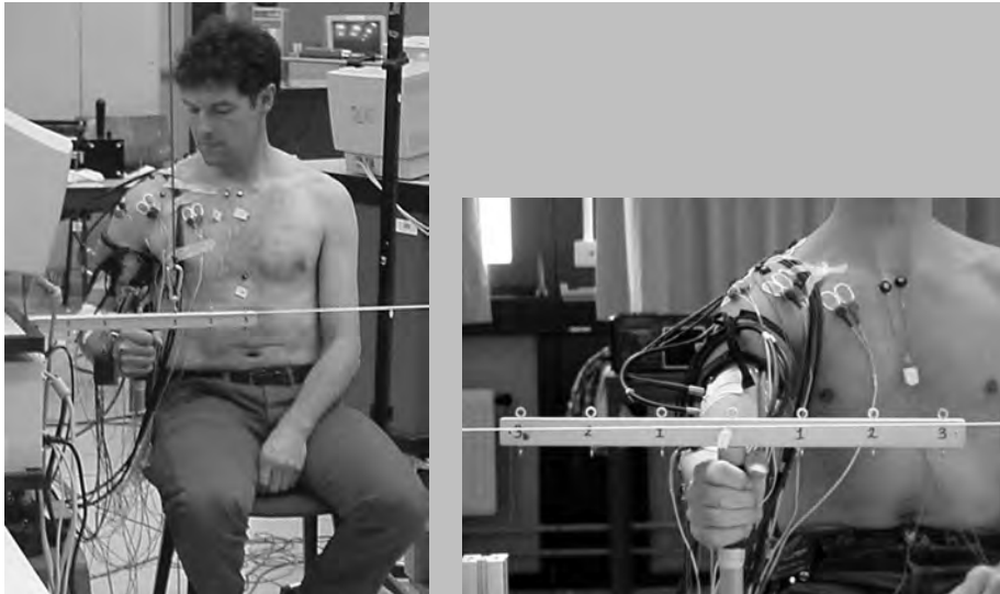
Figure 4.1 Experimental set-up. Subject was sitting on a chair with the elbow flexed and forearm in a horizontal and neutral position. The subject had to hold the tool with his right hand, keeping the bar on top horizontal (a). Visual feedback on the position of the tool was given by a horizontal cord. Flexion moments were enforced by hanging weights right under the stick while extension moments were enforced by loads applied to the middle of the bar using a pulley system. Pro/supination moments were imposed
